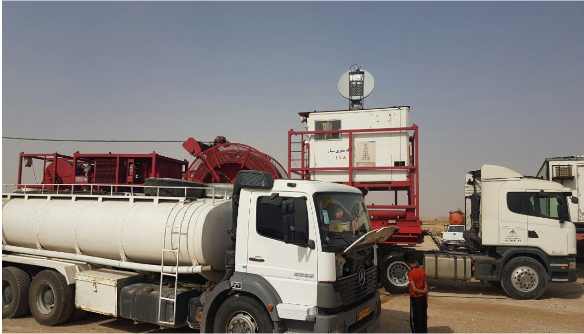
NISOC hub antenna and coil tubing site equipped with auto-deploy antenna
